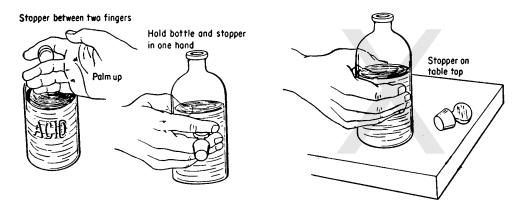
Care must be taken that the stopper is not contaminated while transferring a liquid from a stock bottle.
